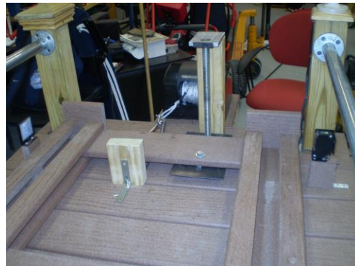
Fig. 15.15. The winch, lift, and release systems.
