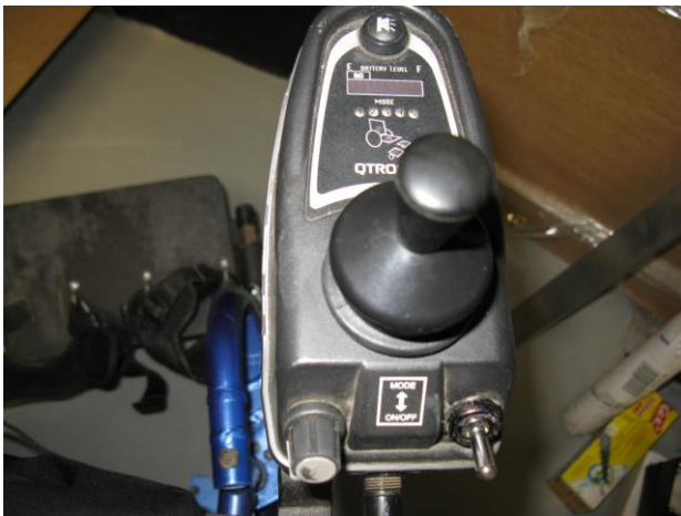
Fig. 15.5. Control mechanisms, incl. joystick (L) and actuation (R).
