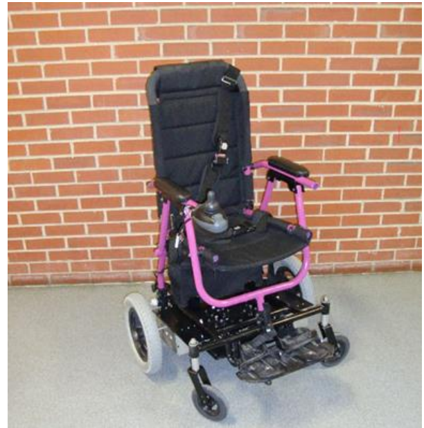
Fig. 15.8. Portable compactable power wheelchair.
