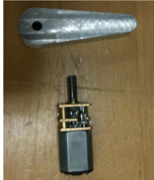
Fig. 15.22. Primary Motor and Swing Arm
